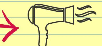
One pole controls the heater, one pole controls the fan, one throw is for low speed, one throw is for high speed
